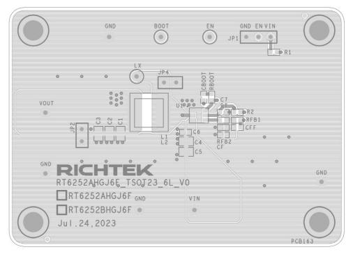
Figure 1. Top View (1<sup>st</sup> layer)
